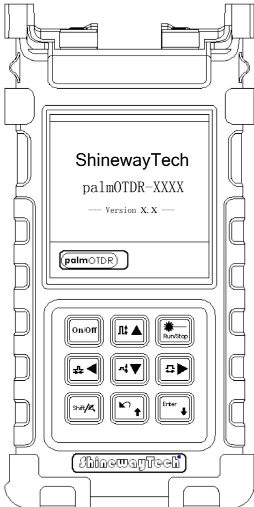
Figure 2-2. Operation Interface of palmOTDR
